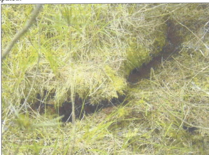
Plate 3.4: A crack in the peat surface beneath forestry which is just visible despite the thick litter layer.
