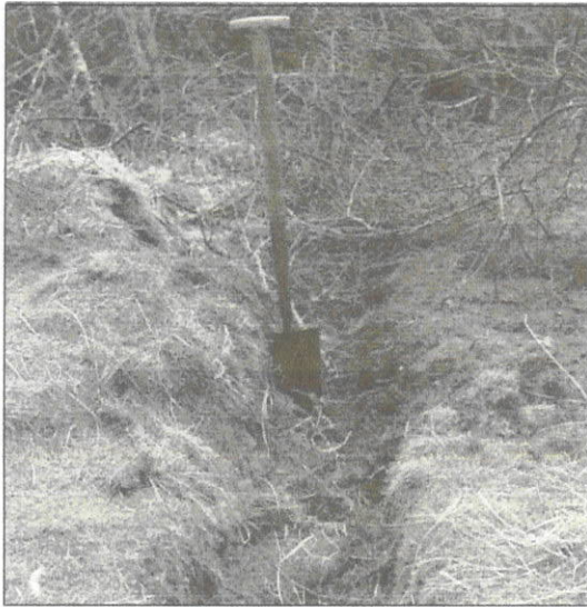
Plate 3.1: Longitudinal crack in a plough furrow under mature forestry on deep peat in the north of Scotland, after removal of the litter layer.
