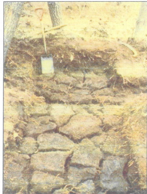
Plate 3.2: Reticulate cracking in a plough ridge under mature forestry on deep peat in the north of Scotland, revealed by removing the surface fibrous layer.
